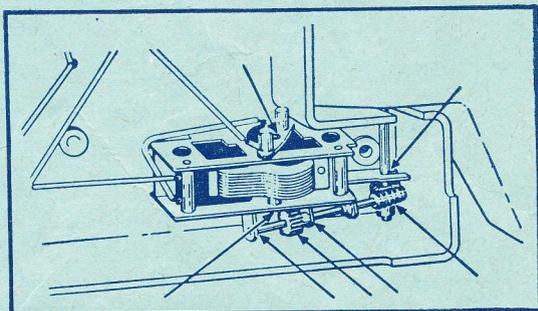
FIGURE 2—LUBRICATE POINTS INDICATED BY ARROWS.
