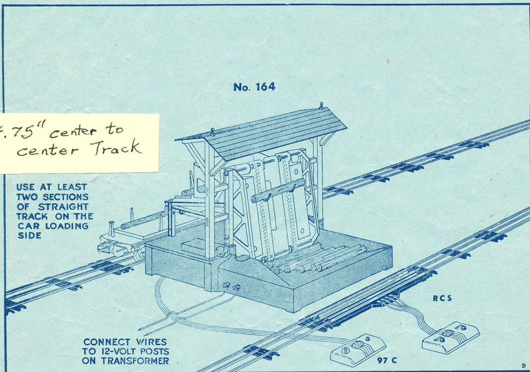
FIGURE 1—PLACE AND CONNECT LUMBER SHED AS SHOWN ABOVE.
