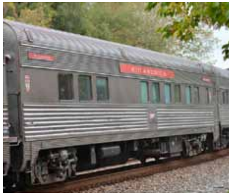
City of Angels (above) is the former New York Central's Laurel Stream with 6 double bedrooms, buffet and lounge built by Budd Co. in 1949.
