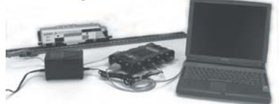
Computer Attaches To TIU RS-232 Port via a 9-Pin Serial Cable
