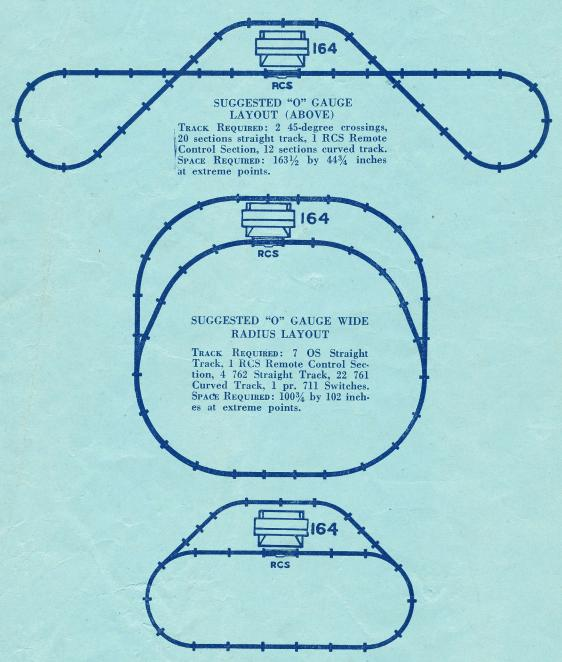
SUGGESTED "0-27" TRACK LAYOUT (Above) TRACK REQUIRED: 14 Sections No. 1013, 13 Sections No. 1018, 1 Pr. No. 1121 Switches, 1 No. 1019 Remote Control Section.
