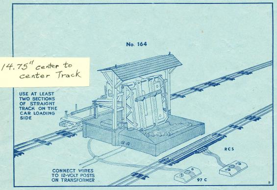
FIGURE 1-PLACE AND CONNECT LUMBER SHED AS SHOWN ABOVE.
